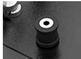
Kit attacco rapido aria compressa sul pianale Quick-release coupling for compressed air on the platform
